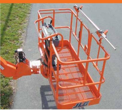
Pipe racks help keep your materials organized and within reach by providing a factory-approved method of storing tubing and conduit in the platform.
