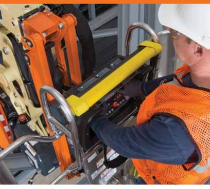
Boom lift operators experience enhanced control panel protection with this aftermarket accessory. When activated by approximately 50 lb (23kg) of force, SkyGuard® stops all functions in use at the time.
