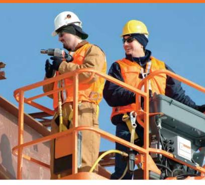
The SkyAir® onboard air compressor delivers 9.3 CFM of air at up to 125 psi—increasing productivity by reducing the risks, costs and hassles of tethering to a separate ground-based compressor.
