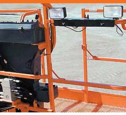
With the Nite Bright® package, you will be able to see your work environment in a whole new light. The package includes two 40-watt lights to illuminate your work site, as well as four 40-watt lights for the area around the chassis. The Nite Bright package is great for low-lit areas such as mines, tunnels and nighttime applications.
