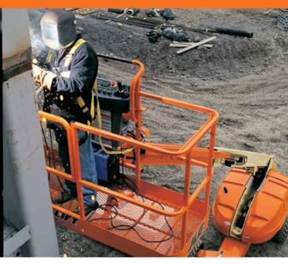
Tucked into the SkyPower® boom platform, the 280-amp Miller® CST™ 280 welder conserves space and provides stick and TIG capabilities. The SkyWelder® eliminates the cost of having a stand-alone welder and power supply.
