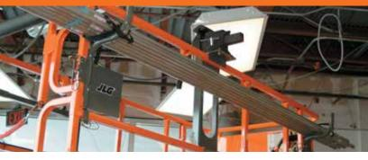
Conserve platform space and reduce trip hazards by storing the materials on the outside of the platform. Pipe racks help keep your tools and materials organized and within reach. Pipe racks come standard with Plumbing, Plant Maintenance and Electrician packages.
